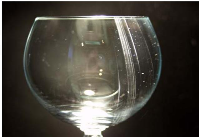
Image 3: Line corrosion
